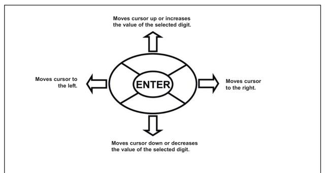
**FIGURE 4-5. Navigation keys.** The operation of the navigation keys is shown. To move a decimal point, highlight it, then press the up or down key.
